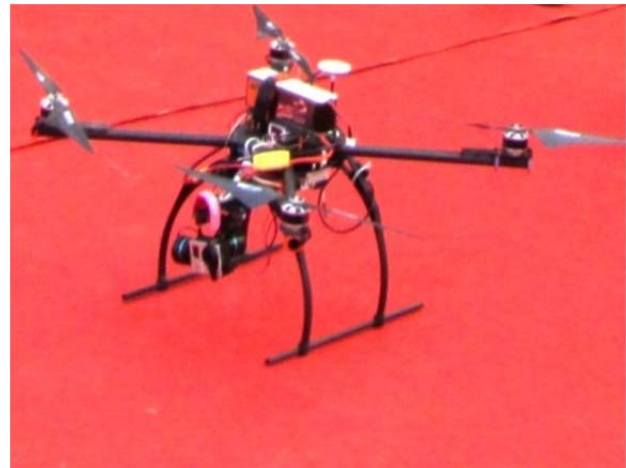
Fig. 1: Quadrotor helicopter and Gyro-stabilized High resolution camera.
